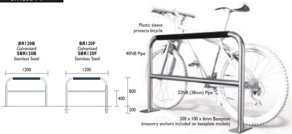
Material Specifications (General)Mild steel40NB (50.0) × 1.5mm Light duty pipe / Hot dipped galvanisedStainless steel40NB (50.0) × 1.5mm Grade 304 stainless steel pipe / Linished finish
