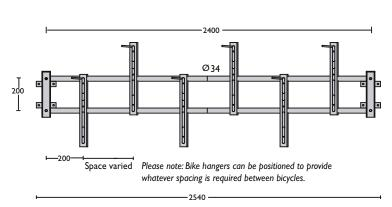
$\label{eq:material} \begin{array}{l} \textbf{Material Specifications (General)} \\ 34 \times 3 \text{mm Beam} \ / \ 60 \times 30 \times 2 \text{mm} \ \ \text{Angle} \\ 19 \ \text{OD} \times 1.2 \text{mm} \ \text{Rail} \ / \ \ \text{Hot dipped galvanised} \end{array}$
