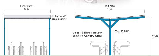
$\begin{tabular}{ll} \textbf{Material Specifications (General)} \\ Frame & 100 \times 50 \times 2.5 mm \ RHS \ / \ Galvanised \\ Roof & Colorbond \ ^{\circ}\ roofing \ sheet \\ \end{tabular}$ Frame Roof
