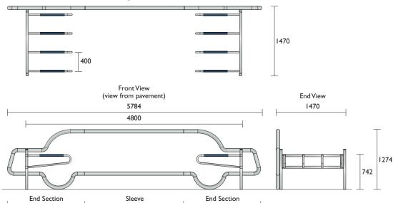
Manufactured in 2 mirror-reversed sections with sleeve straight section
