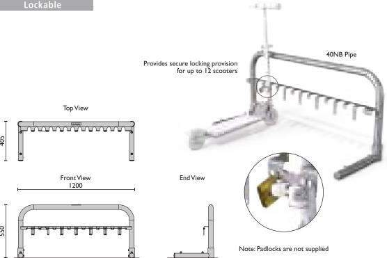
Material Specifications (General)SCR1340NB (50.0) x 1.5mm light duty pipe / Ø12 round bars / GalvanisedSCR12L40NB (50.0) x 1.5mm light duty pipe / Galvanised
