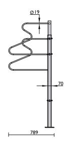
$\label{eq:material Specifications (General)} $70\times70\times2.5 \text{mm Post} / 34\times3 \text{mm Beam} / 60\times30\times2 \text{mm}$ Angle $19\ \text{OD}\times1.2 \text{mm}$ Rail / Hot dipped galvanised}$
