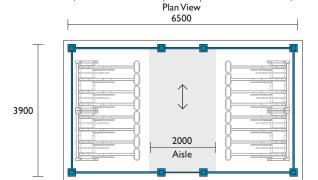
Cage length expanded using modular mesh panels (1500mm wide)
