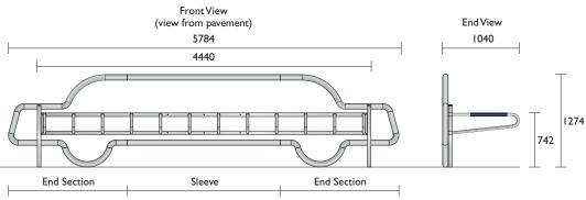
Manufactured in 2 mirror-reversed sections with sleeve straight section
