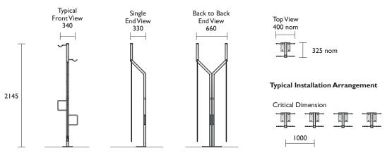
$\label{eq:material_specifications} \begin{tabular}{ll} \textbf{Material Specifications (General)} \\ 50 \times 50 \times 2.5 mm \ SHS / 12 \varnothing \ Rod / 6 mm \ MS \ Plate / \ Hot \ dipped \ galvanised \ PVC \ coated \ steel \ cable \ assembly \end{tabular}$
