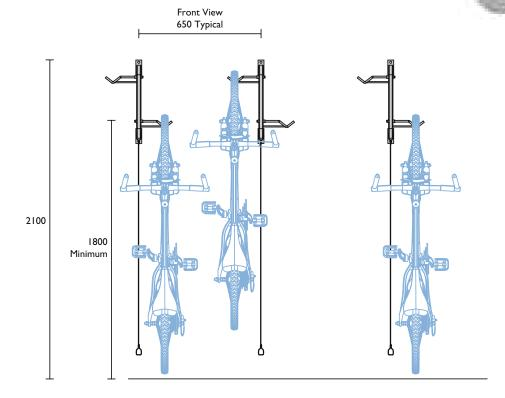
$\label{eq:material} \begin{array}{l} \textbf{Material Specifications (General)} \\ 30 \times 30 \times 1.6 \text{mm SHS} / \text{Hot dipped galvanised} \\ 100 \times 40 \times 6 \text{mm MS plate} / \text{Hot dipped galvanised} \\ \end{array}$
