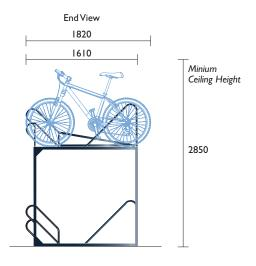
Material Specifications (General)Frame40 x 40 SHS / Hot dipped galvanisedSupports20NB x 1.2mm Pipe / 60 x 35 x 2mm Track / Hot Dipped Galvanised Finish
