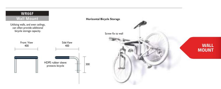
Material Specifications (General)Mild steel8mm Mild steel plate / 40NB (50.0) x 1.5mm / 20NB (25.0) x 1.2mm Pipe / GalvanisedStainless steel8mm Stainless steel plate / 40NB (50.0) x 1.5mm / 20NB (25.0) x 1.2mm Stainless steel pipe / LinishedWR66F20NB (26.9) x 2.6mm Medium duty pipe / Galvanised
