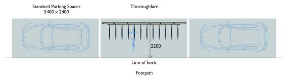
Material Specifications (General) Rack 50 x 50 SHS Mild Steel / 25NB x 1.5mm Pipe / Galvanised Profile
